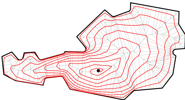
Fig. 12. Cubic B-spline approximation of the polygonal spiral path of Fig. 11(b).
