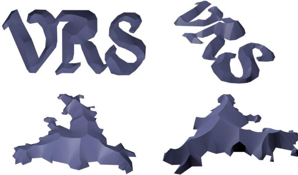
Figure 12: Two different views of sample variable-radius roofs. The roof data was generated by our implementation and then rendered by means of Blender [1].
